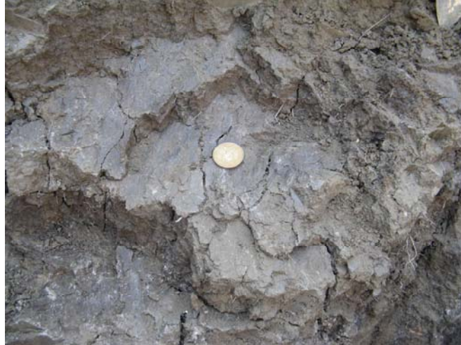
Figure 3. Slickensides in the C ks horizon a Vertisol soil of the Sceptre Association. The glossy pressure faces result from one block of soil sliding by another as the expanding subsoil wets up unevenly. The whitish flecks are gypsum salts, common at about 0.5 to 1 m depth in Sceptre soils. The ‘loonie’ coin provides scale.
